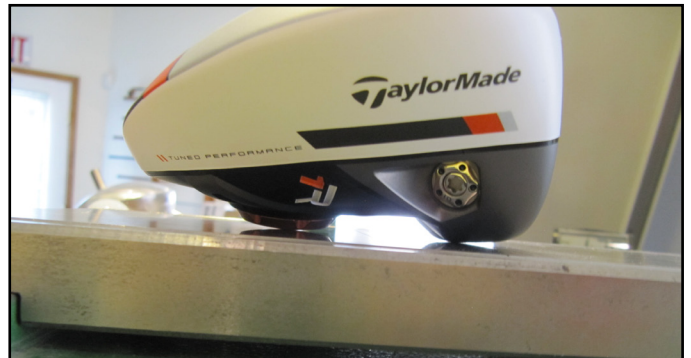
Correct face to back sole touch position for the Taylor Made R1 is defined by the twin touch points of the front sole and the rear protruding adjustable sole piece
